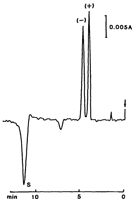
FIGURE 24. Liquid chromatographic resolution of (+/-)- N -t-BOC-phenylalanine using an ion interaction agent. (From Pettersson, C. and Shill, G., J. Liq. Chromatogr. , 9, 269, 1986. With permission.)
